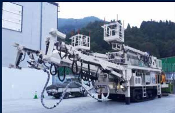
Real-Time Sprayed Concrete Thickness Measurement System
