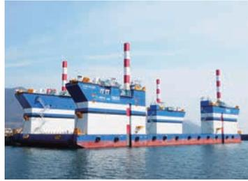
Semi-submersible spud barge (Float Raiser)
