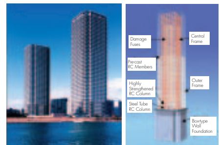
W-Comfort Towers (WCT) Structural Model of WCT
