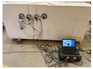
(2) Surface Water Absorption Test
